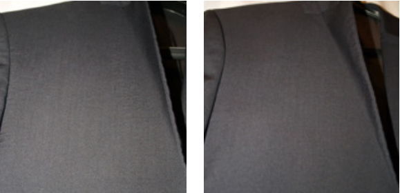
Figures 6 and 7: Examples of the different results after finishing on a form finisher, prior to ironing. After 3 cleaning and drying cycles. Strong appearance of bubbles and wrinkles on the left; very limited appearance of bubbles and wrinkles on the right (all removed after ironing)
